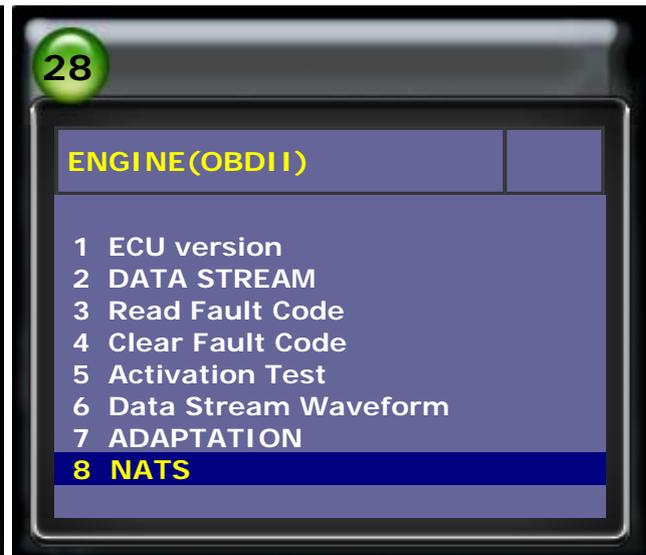
14. Key registration will clear all key entries. It is necessary to register all the keys. Non-registered key can not start the engine.
